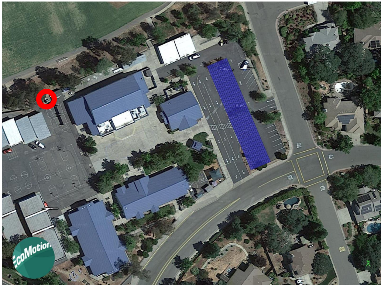
Sample PV Layout showing 149 kW
